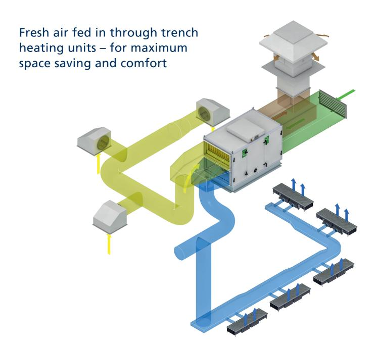
Almost all **Katherm trench heating units** can be fitted with a **supply air function** for specific projects. Primary air, pre-conditioned by a central ventilation unit, can be introduced into a room through various supply air spigots, perfectly combining heating, cooling and a supply of fresh air. The space requirement is thus minimised and comfort in the building maximised.
