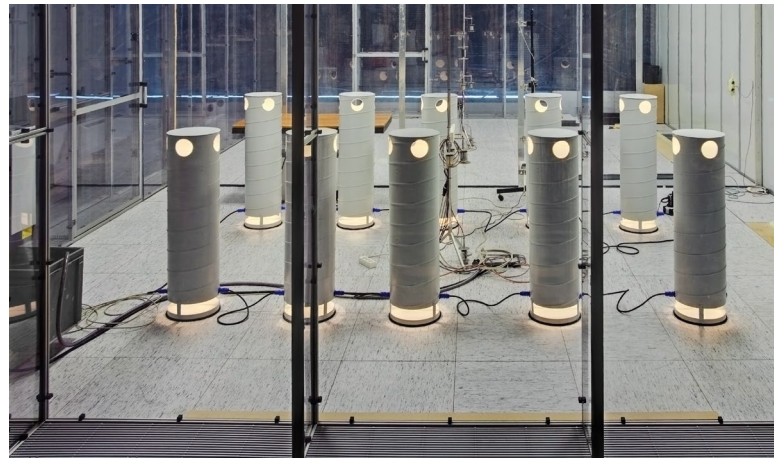
Heat and cooling output test cabin
