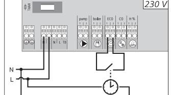
The base station is equipped with an ECO input for connecting an external timer, if the internal clock of the room control unit Radio Display shall not be used. When the input is activated by the timer, the heating zones are switched to night operation.
