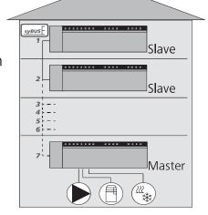
**Note:** The base station the components are connected to must be configured as master. Further base stations can only be paired with the master base station.
