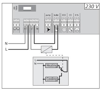
If no external change-over signal is available, the internal pilot function of the base station can be used for switching the overall installation between the operating modes Heating and Cooling. A relay used by the base station for switching over is used for this.
