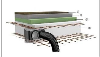
① Concrete ceiling ② Footfall sound insulation ③ Screed ④ Floor covering
