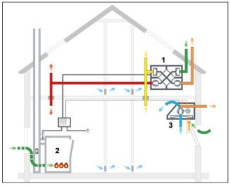
1 Ventilation unit positioned centrally, for the entire apartment, supply and exhaust air unit with or without heat recovery
