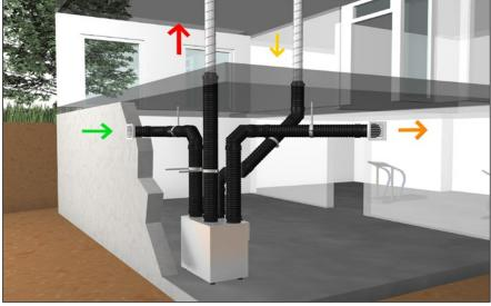
Outside and outgoing air lines with the heat-insulated MAICOTherm ventilation duct system.
