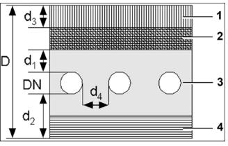
1 Screed 2 Insulation 3 Concrete slab with ventilation duct 4 Filigree flooring
