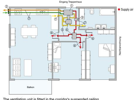
The ventilation unit is fitted in the corridor's suspended ceiling
