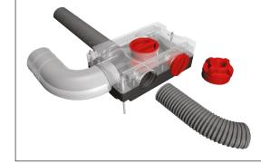
Ensure that the ducts are insulated in line with the relevant standards. To prevent condensate from forming, especially in outside air and outgoing air ducts carrying cold air inside heated rooms, the insulation must prevent vapour diffusion and/or duct systems with protection from vapour diffusion (MAICOTherm) should be used.
