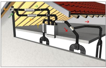
Use of a KWH ... L/R combi-wall connection as an outside and outgoing air opening.
