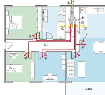
Air flow with patented zone control for supply air / zone 1 = zone 2 =
