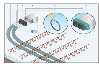
Lubricant should be used when fitting the <u>MF-FDR gasket</u>. The <u>MF-WE slide-in adaptor</u> should be affixed to the <u>MF-W bracket</u> using adhesive tape.
